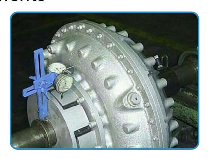
The dial indicator or the dial gauge is one of the simplest and the most widely used Mechanical comparator.
