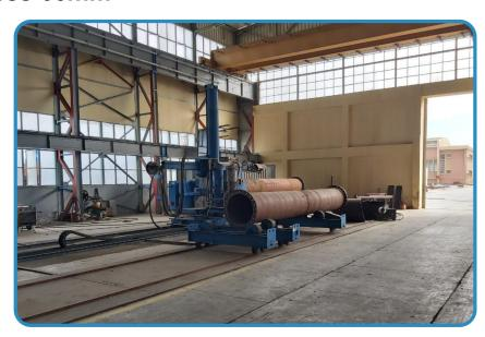
Welding process facilities: Manual welding Submerged Arc welding Gas metal arc welding Argon welding
