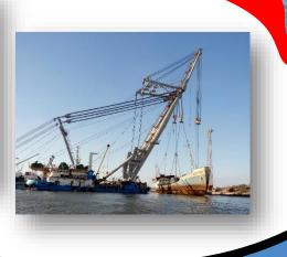
Floating cranes Two salvage floating crane (sheer leg) ENKAZ I & ENKAZ II Wing capacity 500 ton on main hook
